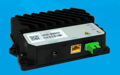
Meet everyone's bandwidth demands with Hitron's NOVA-2000 10G xPON ONT/ONU. This powerful solution delivers speed up to 10 Gbps\* downstream and 10 Gbps\* upstream based on a 10 Gigabit PON fiber interface (EPON or XGS-PON). You can deliver ultra-high symmetrical bandwidth for business customers, as well as premium tier residential services to meet the most demanding HD and ultra-HD video on demand, cloud gaming, multi-Gigabit data, telecommuting applications and more.
